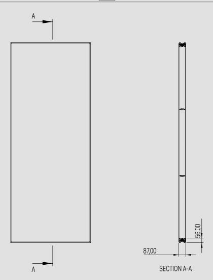
**STRUCTURE:** supporting structure in extruded aluminium on 4 sides.
