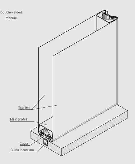
**PERPENDICULAR DIMMING:** from 100% to 20% (depending on the fabric used).
