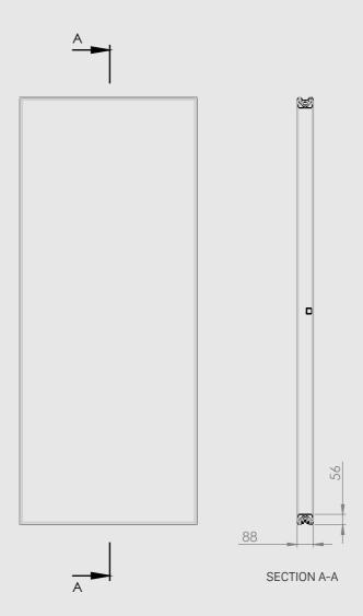
**STRUCTURE:** supporting structure in extruded aluminium on 4 sides.
